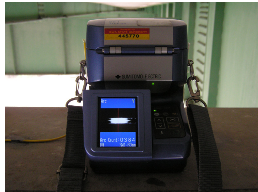
d. Fusion splicer during the arcing process
