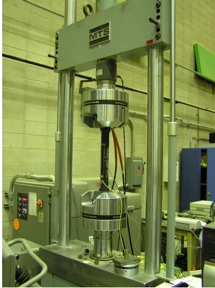
Figure 3.3. Photograph of Coupon A and testing frame used in CT1.
